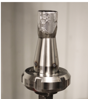
Cone spot welded to the welding sleeve
