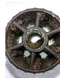
Fig. 2 Picture depicting MBBR reactor and Picture depicting biofilm formation on carriers
