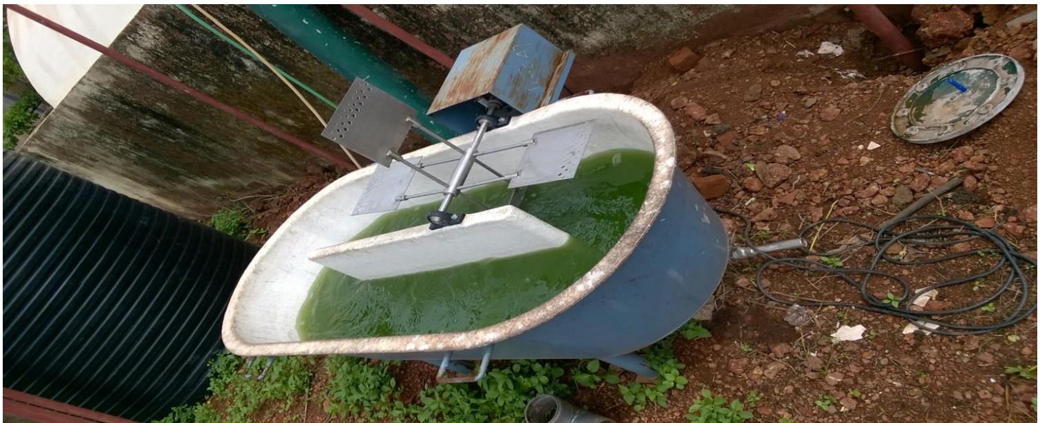
200 Litre capacity microalgae cultivation
