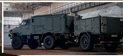
The ŻUBR vehicle in the BYSTRA version is designed for detecting and designating targets in short-range anti-aircraft systems used for tactical protection of combat formations against air attack means. This vehicle is a multifunctional and multi-tasking radar with of detecting and tracking typical threats such as combat aircraft and helicopters, missile projectiles, unmanned aerial vehicles, and mortar shells
